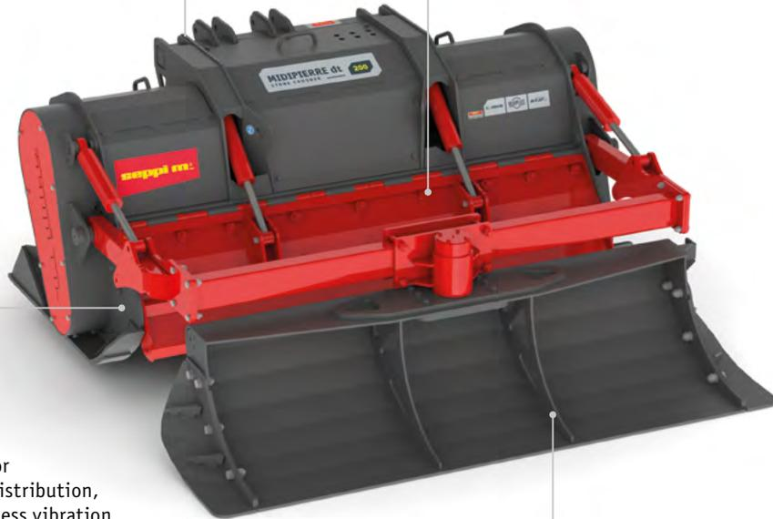
Grader blade (option), hydr. height and rotation adjustment, with hydraulic pneumatic damping incl. lateral extensions
