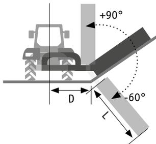
The boom can be angled 90 ° upwards and tilted 60° downwards
