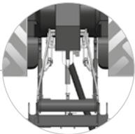
Option: Safe and comfortable connection with PENTALINK stabilization system
