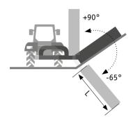
The boom can be angled 90° upwards and tilted 65° downwards
