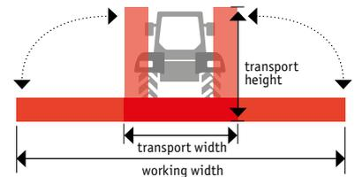
Each single mulcher can be folded up for transport and parking.
