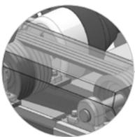
STOPSAFE™ safety system, stops the rotor when the wing mowers are lifted
