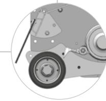
Due to the close position of the roller to the rotor, the rotating flails clean the roller, and the cut material is evenly distributed over the top.
