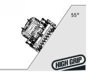
Stability and grip of the vehicle on difficult terrain up to 55° slopes, under optimal conditions
