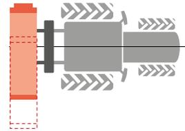
The power belt chassis is very compact - it allows the machine to work under low canopy close to the trunk
